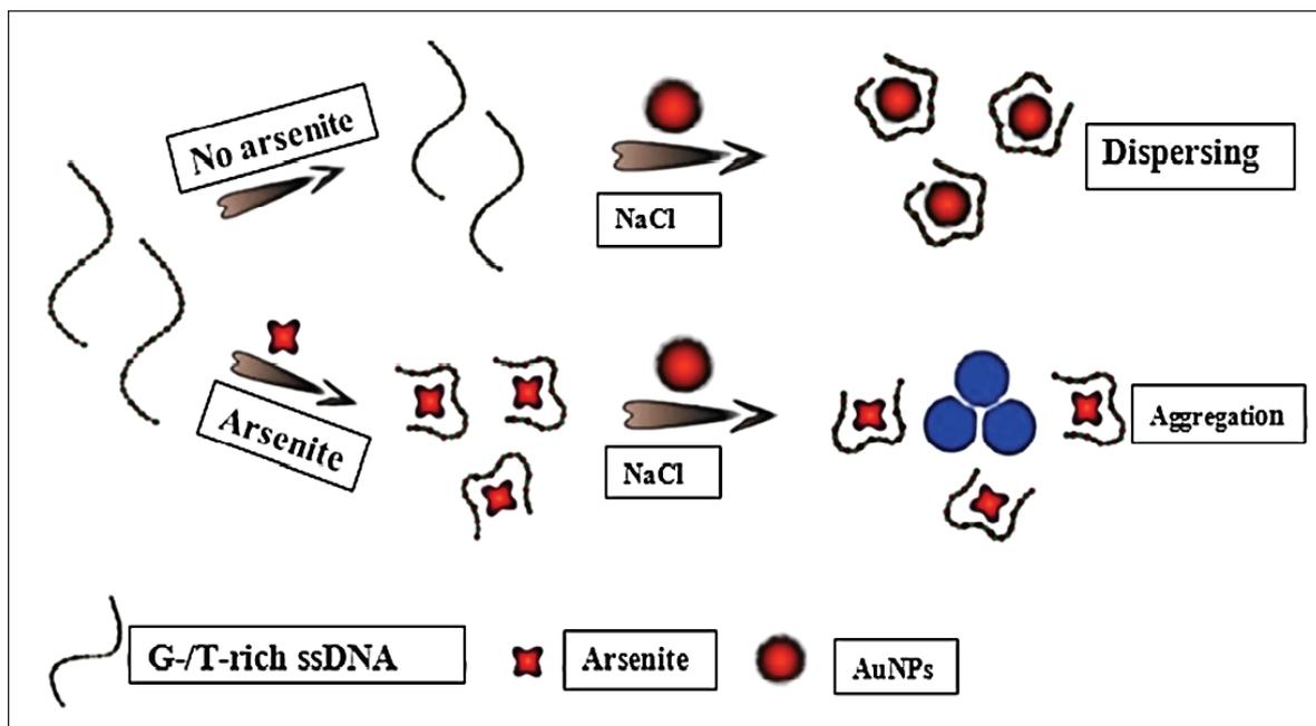
Fig. 8. AuNPs-based colorimetric strategy for arsenite detection [63]
