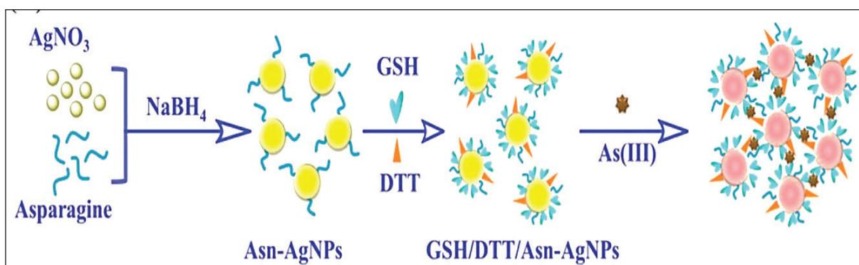
Fig. 2. Illustration of synthesis of GSH/DTT/Asn-AgNPs used as a colorimetric probe for As (III) detection [52]
