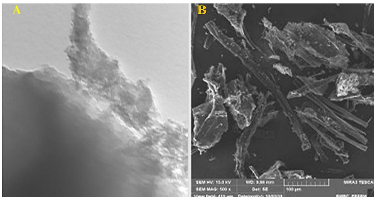
**Fig. 2.** A) TEM of the Cu-NW-AC B) SEM images of the Cu-NW-AC
