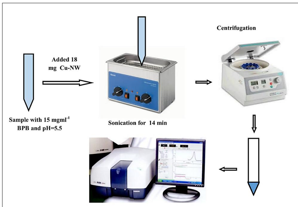
**Fig. 1.** The steps of adsorption and measurement of BPB
