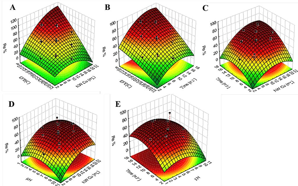
**Fig. 3.** 3D response surface plots for investigation of the effects of different factors on removal of BPB dye removal using Cu-NW-AC adsorbent
