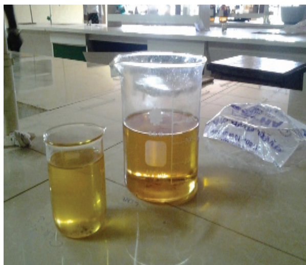
Fig. 1a. Low FFA oil after acid-catalyzed esterification
