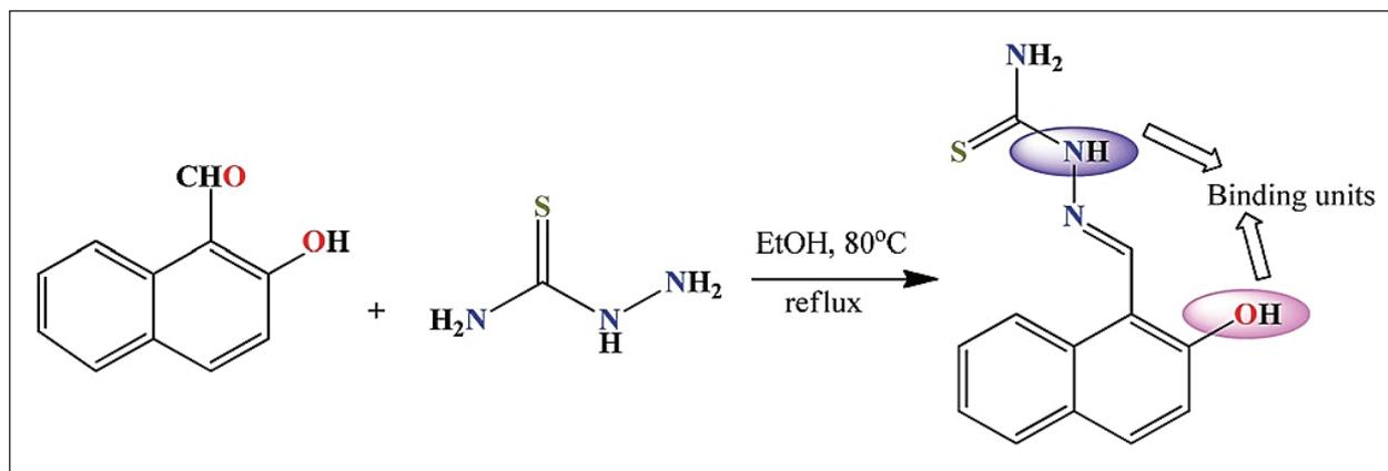
**Fig. 11.** Diagram of the synthesis of the probe for the detect arsenite and cyanide ions [69]
