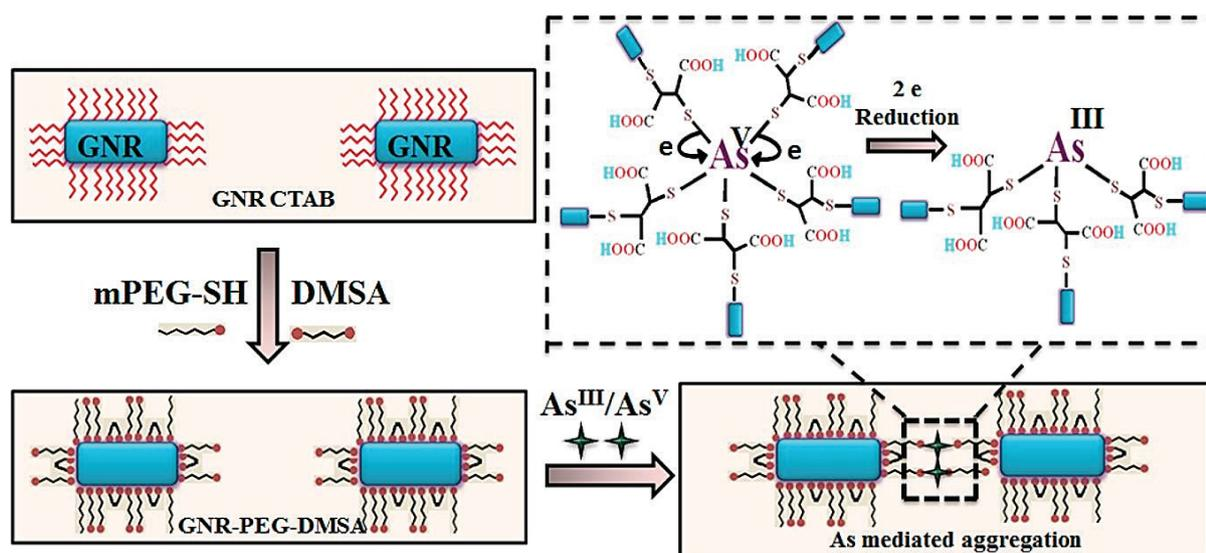
Fig. 3. Illustration of the fabrication of GNR-PEG-DMSA sensor and its interactions with As (III) and As (V) [55]
