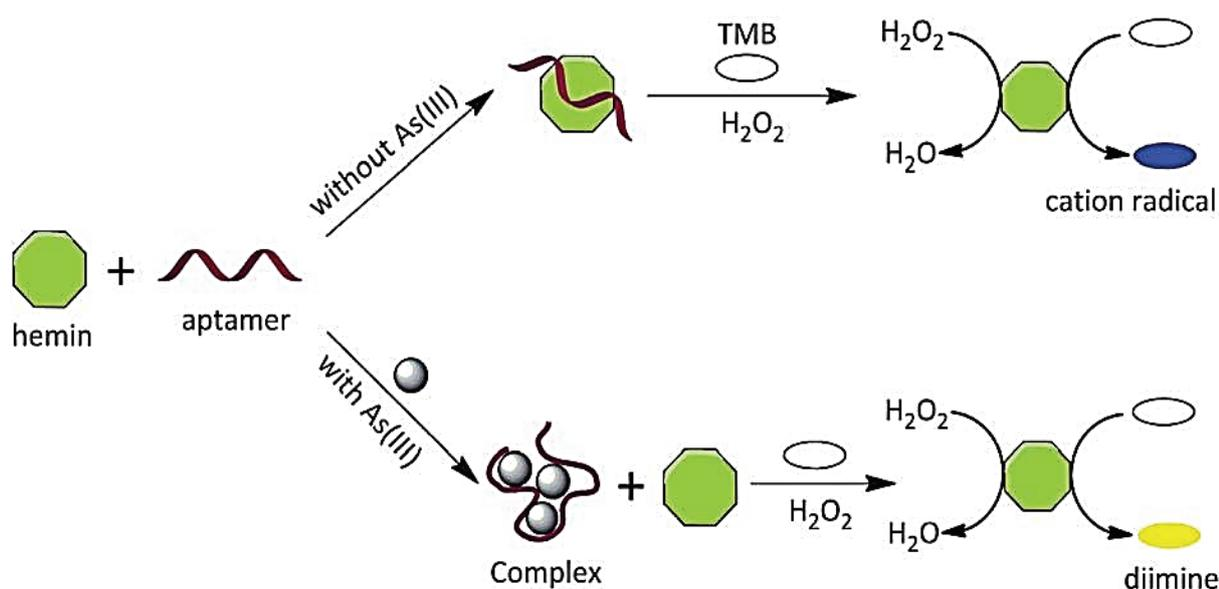
**Fig. 1.** Schematic description of the colorimetric detection of As (III) based on the inhibition of hemin peroxidase activity by arsenic-binding aptamers [33]
