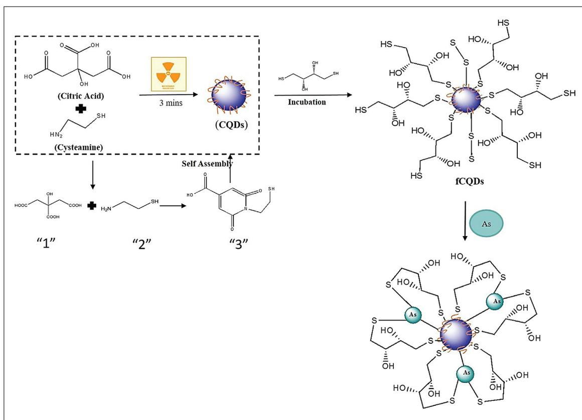
**Fig. 12.** Schematic representation of the synthesized DTT functionalized CQDs for detection of arsenite and binding mechanism of arsenite [77]
