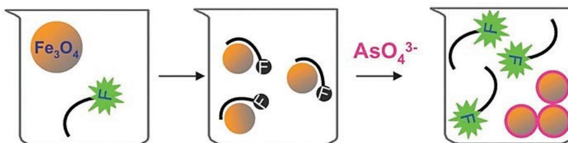
**Fig. 20.** Illustration of sensing arsenate by DNA functionalized iron oxide nanoparticles [94]
